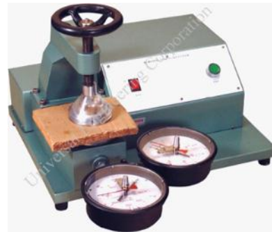
Burst tester for paper
