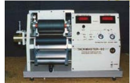
Tackometer :accurately test ink tack.
