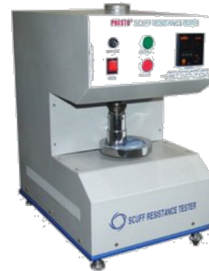
Scuff resistance tester for quality of adhesion with substrate
