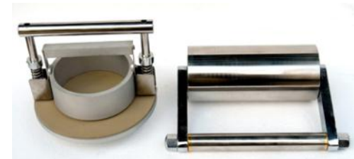
COBB tester for testing water absorbency for paper
