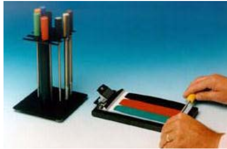
Draw down tester for Ink shade (L*a*b*)
